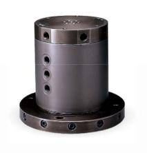
Double rotary type combines two rotaries on same axis to keep the overall height lower still. Two types are available with 12 or 16 circuits, and each circuit can be used independently.
