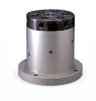
Rotary joint model WRB was developed for low pressure applications. Aluminum is adopted as body material to reduce the weight. This is a center through type, which the through bore of rotary shaft can be used for coolant piping.
