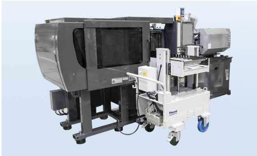
2,500kN (250ton) Two-color IMM Horizontal loading Mold changer : Powered, Drive rollers type
