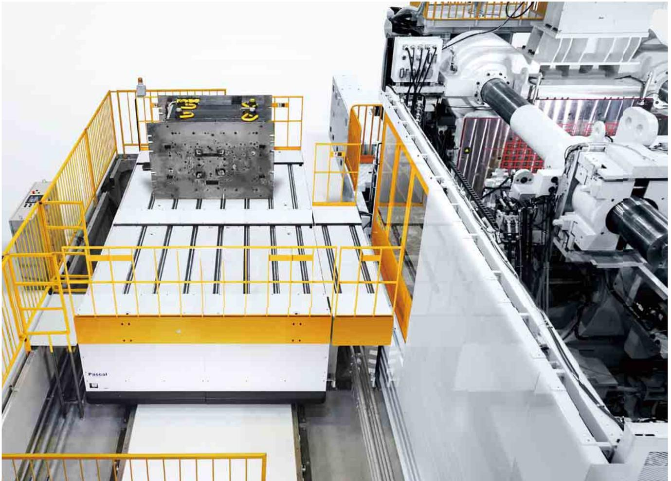
30,000kN(3,000ton) IMM Horizontal loading
