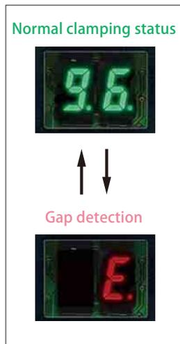
As for DD mag clamp, the status indicator is added to the control box.
