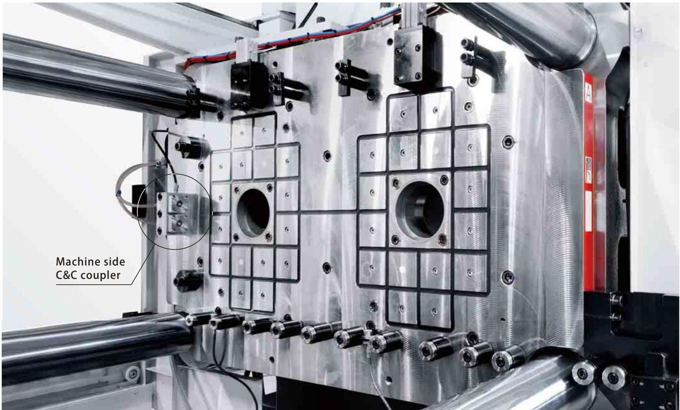
2,500kN (250ton) Two-color IMM Horizontal loading Fixed side Mag clamp & C&C coupler
