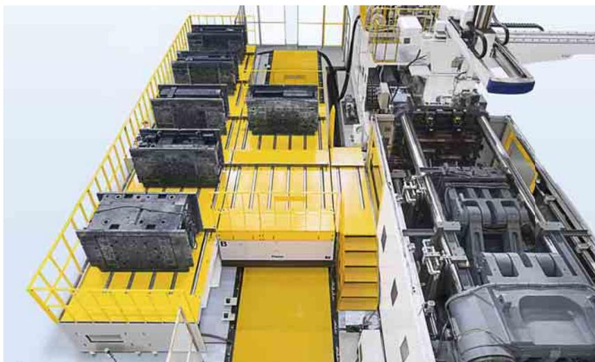
4,500kN (450ton) IMM Horizontal loading Mold changer : Powered, Drive rollers type
