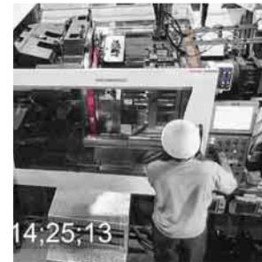
The moving picture of mold change operation for two-color IMM with mag clamp is being uploaded in Pascal web site.
